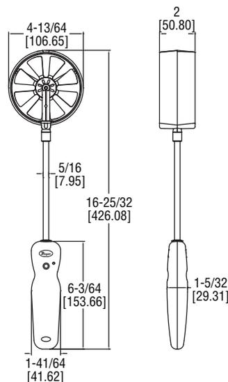
The Model VP2 Wireless 100 mm Vane Thermo-Anemometer Probe measures air velocity, air flow, humidity, and temperature when combined with Models UHH and UHH2 or the Dwyer Mobile Meter app. By having a larger diameter, the rotating vane is able to measure velocities down to 50 fpm or 0.25 m/s. An arrow is molded into the vane housing to depict the flow direction.
